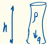
Pressure at bottom of hydrostatic column
